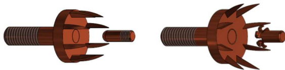
Fig. 12. Sketches of cathode - anode system before explosion (left) and after explosion (right). The cathode-anode system as part of the unit is shown in the sketch, see Figure 4.
